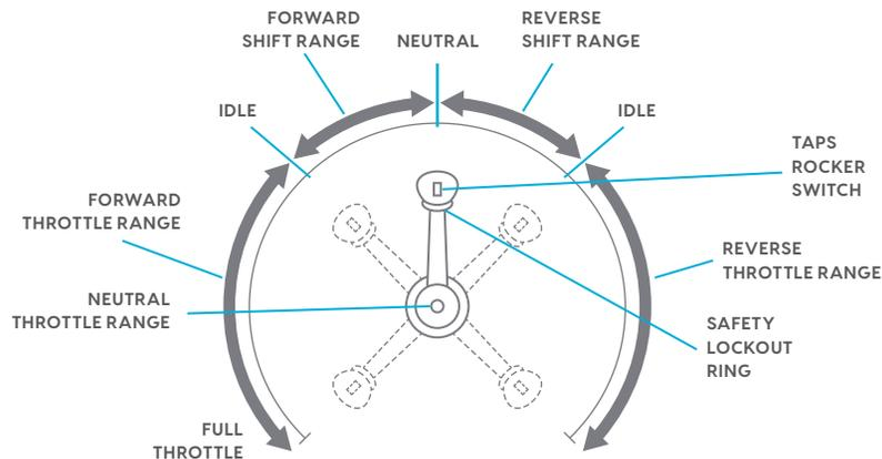
To “rev” the engine without engaging the transmission from NEUTRAL, push in the neutral throttle button and advance the throttle handle. To return to normal operation, return the throttle to the NEUTRAL position.
