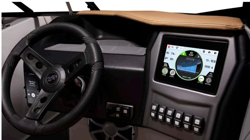
**FUEL GAUGE:** Indicates the approximate amount of fuel in the tank. The ignition switch must be in the RUN position to activate the gauge.
